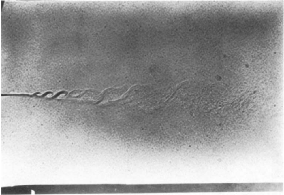
FIGURE 4. Shadowgraph of mixing layer in flow between nitrogen (upper) at 326 \text{ cm s}^{-1} and air at 123 \text{ cm s}^{-1} . Pressure = 7 atm.
